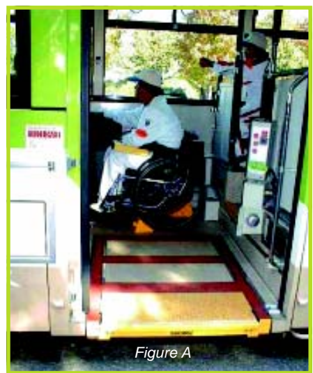
Figure A (above) shows an example of AD products. This type of bus leans when it stops and, thus, has no steps to climb. Older persons, children, and persons on wheelchair can easily get on and off.
